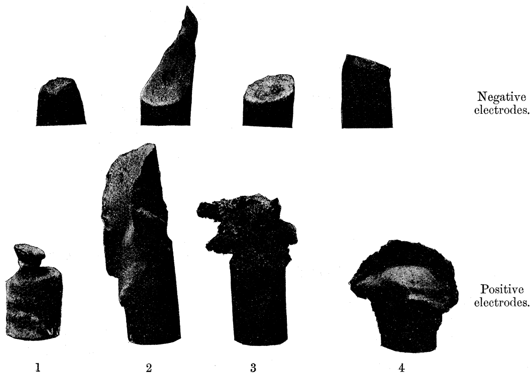
Fig. 9. Photograph of carbon electrodes after use. (Horizontal arc.)
